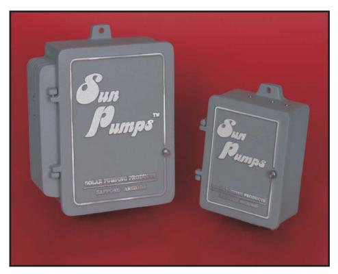
**SunPumps** PCA and PCB series pump controllers are high quality, micro-processor controlled DC power converters designed as the interface between a DC powered pump and the power source. The DC source may be solar modules, batteries or systems using wind generators. The main purpose of a PC series controller is to maximize the total daily water delivery while providing protection for the pump as well as the power source.
